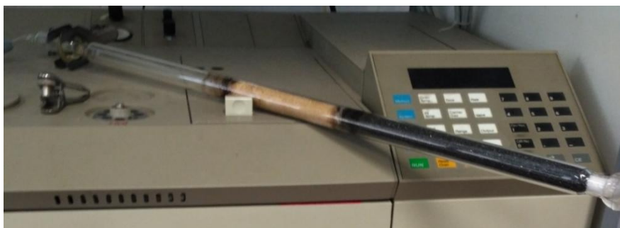
Figure 15 - Reactor with inert material and raw biomass sample
