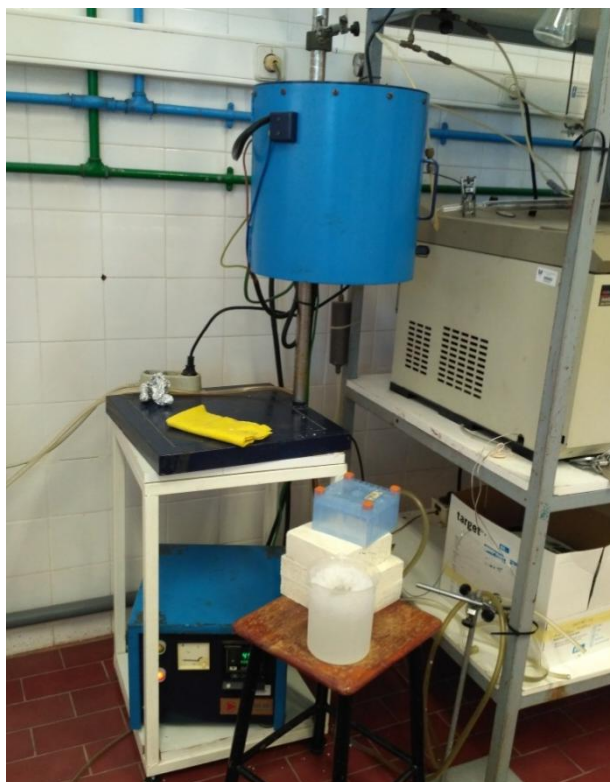
Figure 14 - Fixed bed vertical reactor used for pyrolysis
